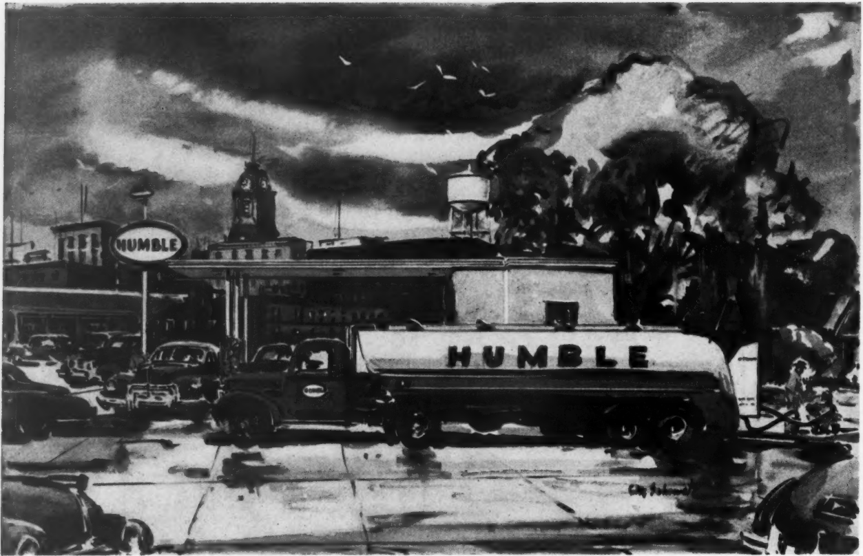
BIG TRANSPORT TRUCKS deliver gasoline directly from terminal loading racks to retail stations in cities and towns. Dumps of 4,600 gallons or more are made into large underground storage tanks, minimizing safety hazards by reducing public contacts at delivery times.
